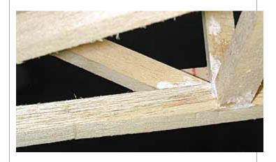
10 By increasing the gluing area that holds the joints together, these 1/32-inch gusset plates add strength to an already strong fuselage structure.
