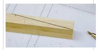
3 Cut the diagonal splice with a band saw, and make sure the cut is square to the top edge.
