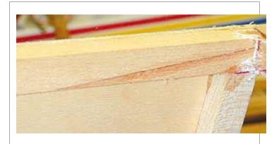
9 Here you see the splice positioned close to a cluster junction where other fuselage members join.
