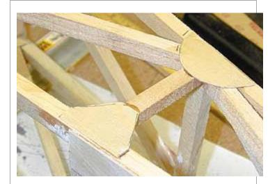
11 This is a close-up of an internal gusset plate used to strengthen a lower fuselage longeron. These are used when you want a flush outer model
