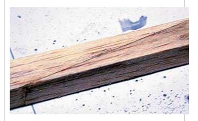
8 For additional strength, I positioned the splice against the plywood side sheeting.
